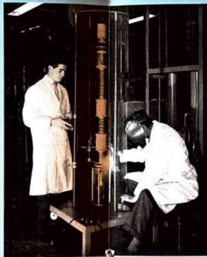
One of the last stages of assembly of a high-power Klystron. The English Electric Valve Company has supplied this type of Klystron for many important applications in the field of communications and radar, and the latest of these is used in the output stages of the new BBC-2 transmitters
