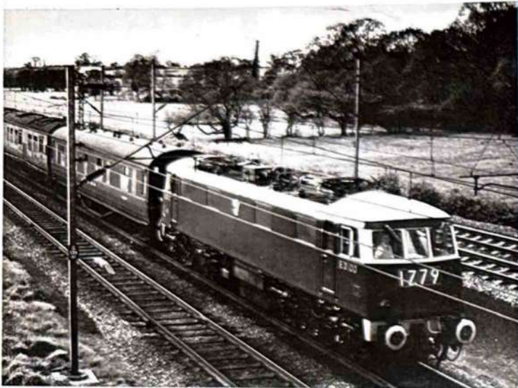
A 3,000-h.p. 25-kV a.c. electric locomotive fitted with transducer control equipment developed by English Electric to give greatly increased adhesion characteristics
