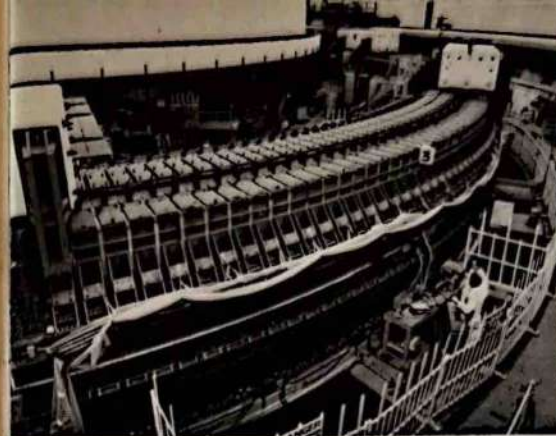
The GeV proton synchrotron "Nimrod" at the Rutherford High Energy Laboratory, Chilton, Berkshire. Two scientists carrying out a survey of the magnetic field of one of the octants of the 7,000-ton electro-magnet which holds the protons in their orbit as they are accelerated
