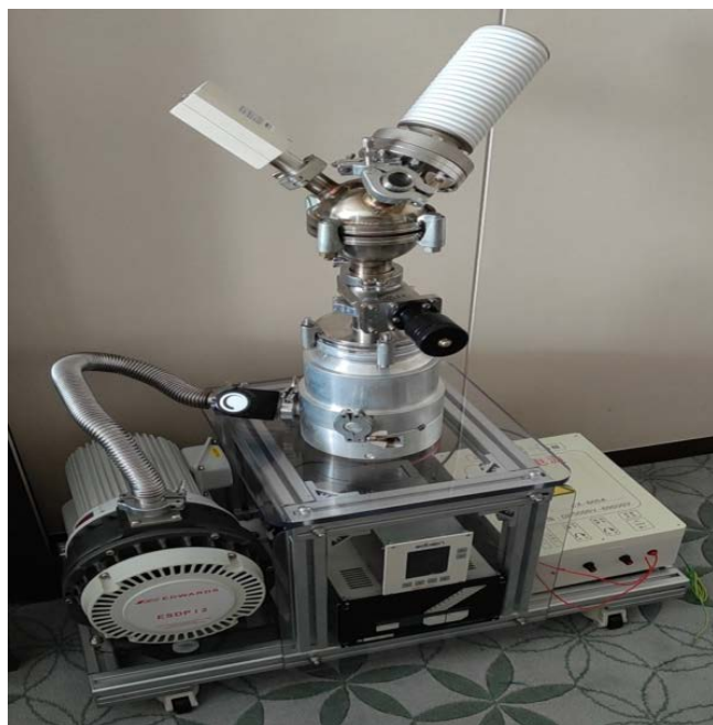
Figure 2. Picture of own-made fusor.
