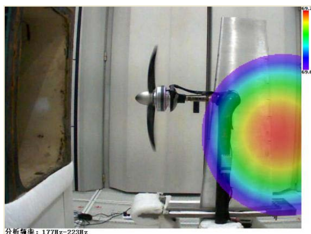
Fig. 8 Sound source location at different relative positions at wind speed of 30m/s
